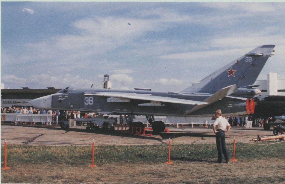
An Su-24M at Khodynka in 1989. This particular aircraft differed from earlier Su-24Ms in that it lacked the large wing fence usually found on this type and is intended for export. (Nick Cook)
