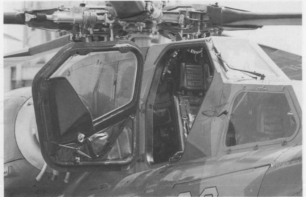
A view of the pilot's station with the armored door open. The panel at the front of the door is armor, a reminder of the lessons of the Afghanistan war.
