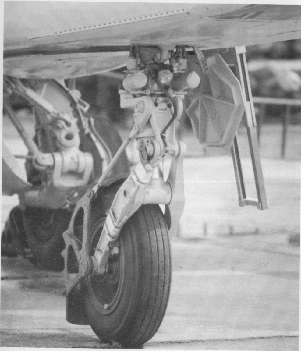
▲ A close-up view of the front landing gear. The anti-FOD debris catcher at the rear of the wheel is finished in dark green, as is the wheel hub.
