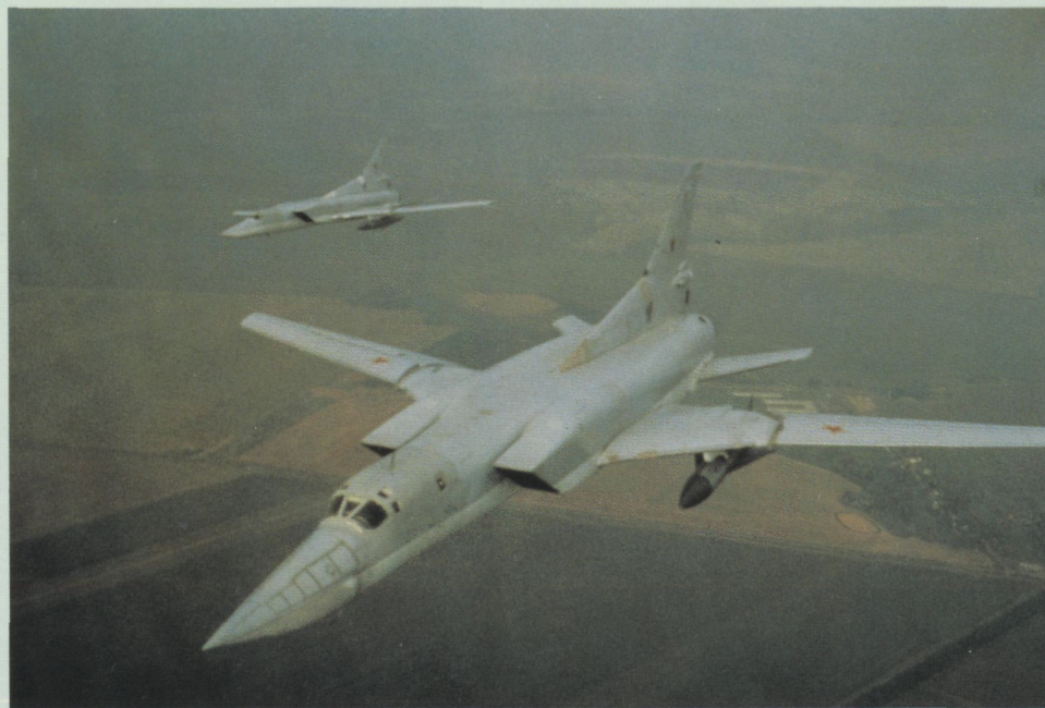
A pair of Tu-22M3 Backfire Cs on a peacetime exercise, armed with K-26 missiles. This type of aircraft is categorized by the Soviets as a Raketnosets -Missile-carrier, rather than as a bomber. (Sovfoto)
