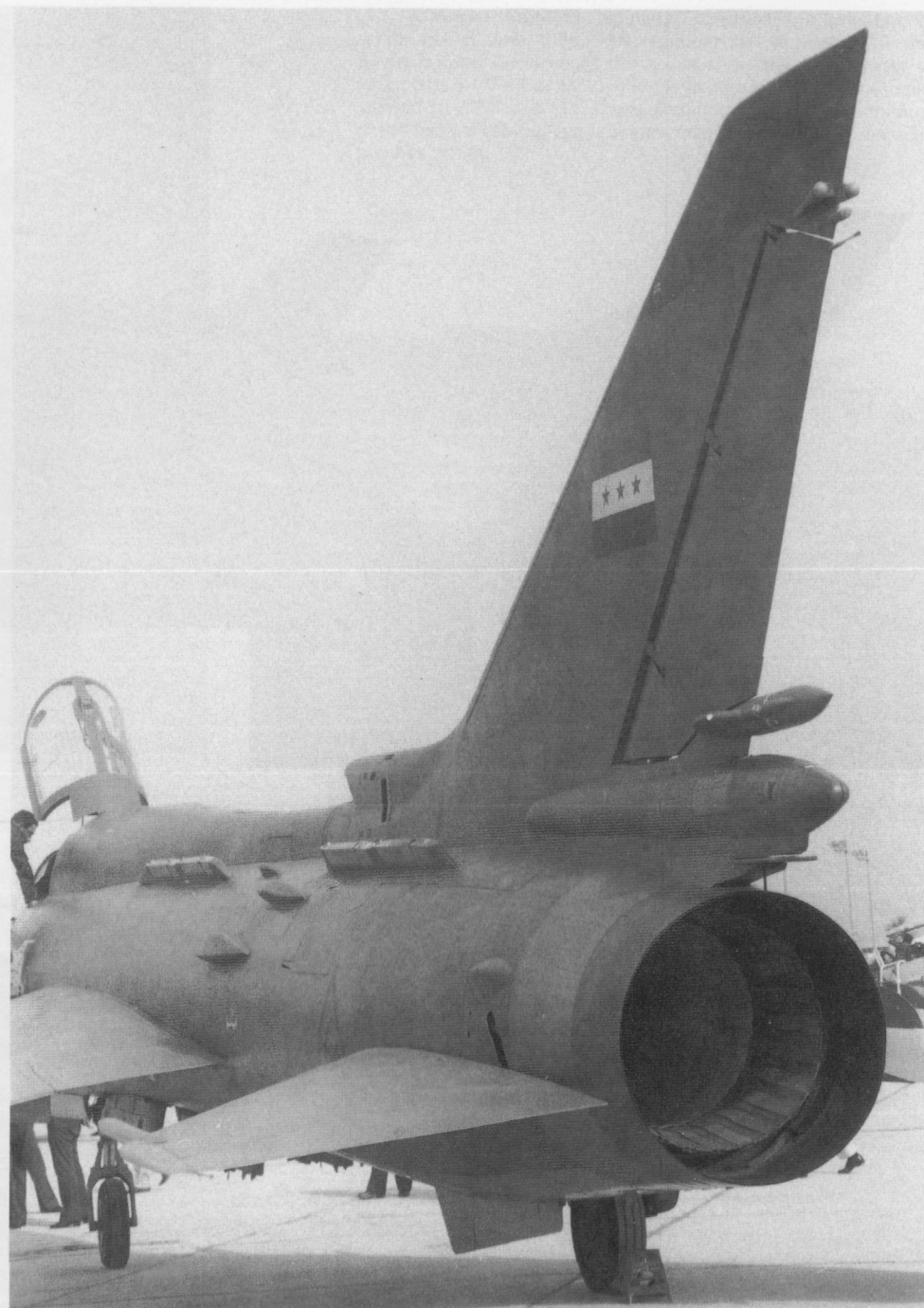
A view of the rear of the Su-22M4 fuselage, showing the exhaust pipe of the Lyulka/Saturn AL-21F3 engine. (Christopher Foss)
