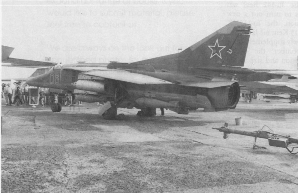
The MIG-27KR is the latest attack version of the Flogger family. It is most readily distinguishable by its longer nose and the oval optical port at its tip. This particular aircraft was exhibited at the Central Frunze Air Base at Khodynka in August 1989.
