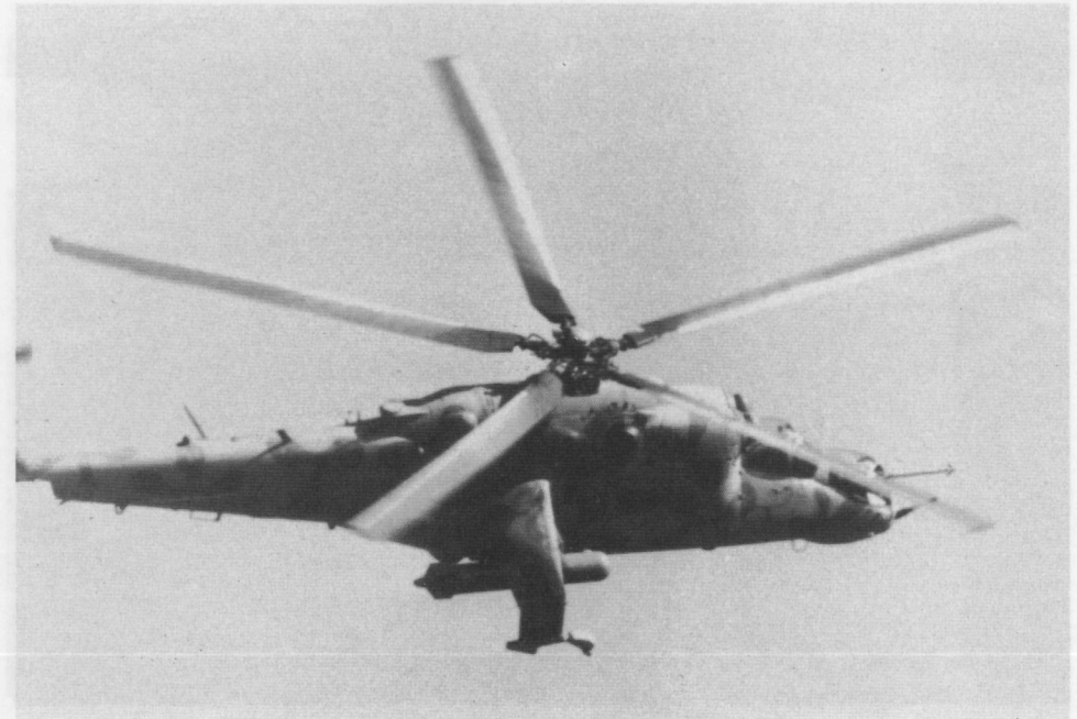
This overhead view of a Mi-24R Hind G shows the stub winglet attachment points which characterize this variant, and also show the uncommon 350 liter drop tanks.
