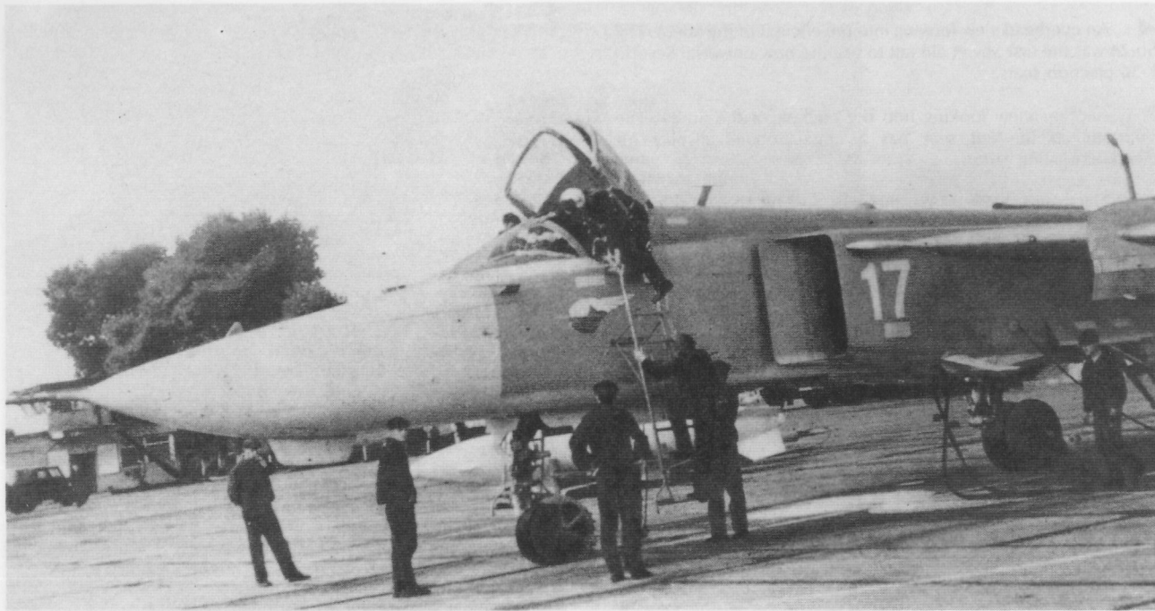
The Su-24MP Fencer F, an electronic warfare variant of the Su-24 series. It is identifiable by the antenna under the nose and the sickle shaped antenna barely evident under the number (17) on the lower edge of the fuselage side.
