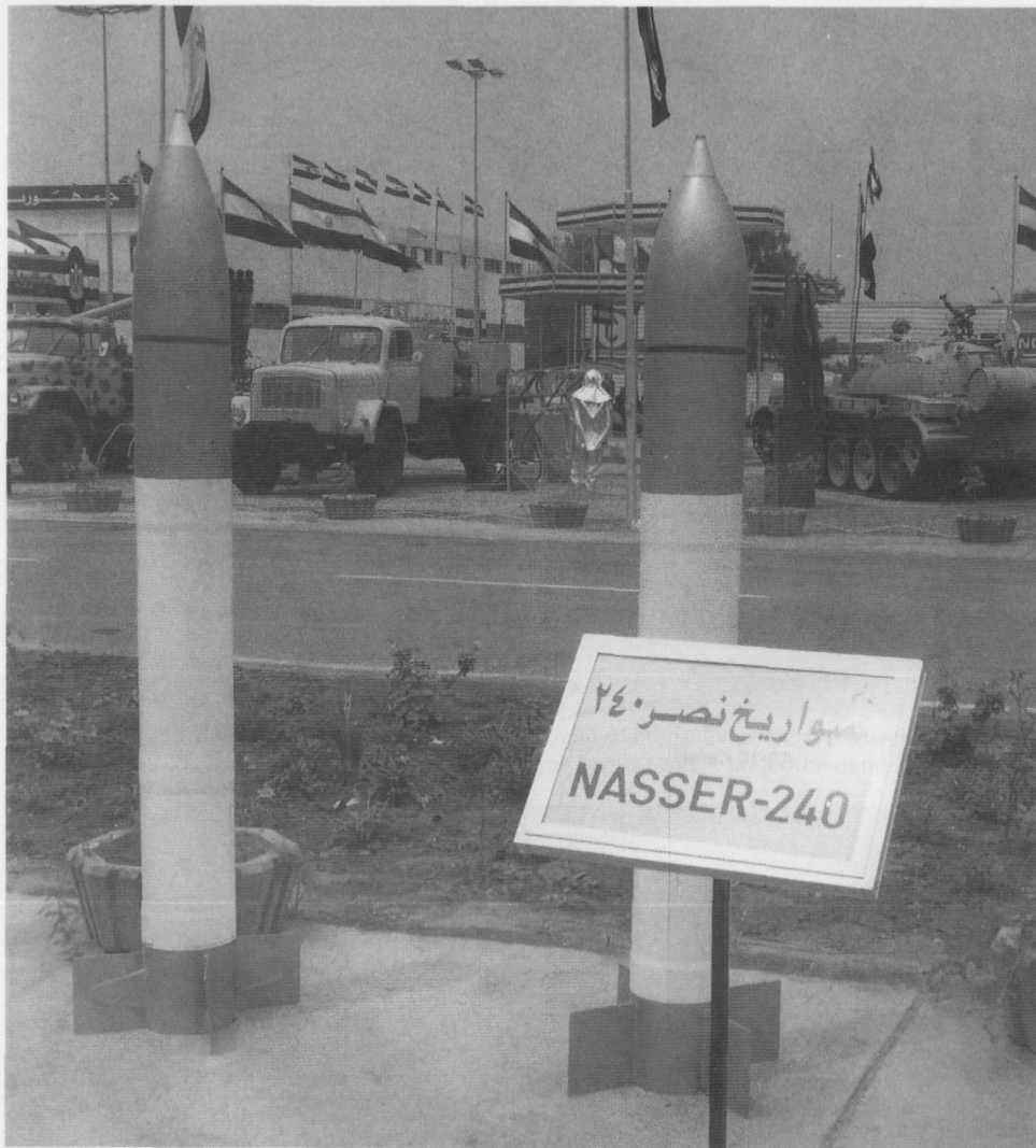
The S-24 is a large 240mm diameter unguided rocket fired from Soviet attack aircraft. This view shows a pair of S-24 of Iraqi manufacture, called the Nasser 240. (Christopher Foss)
