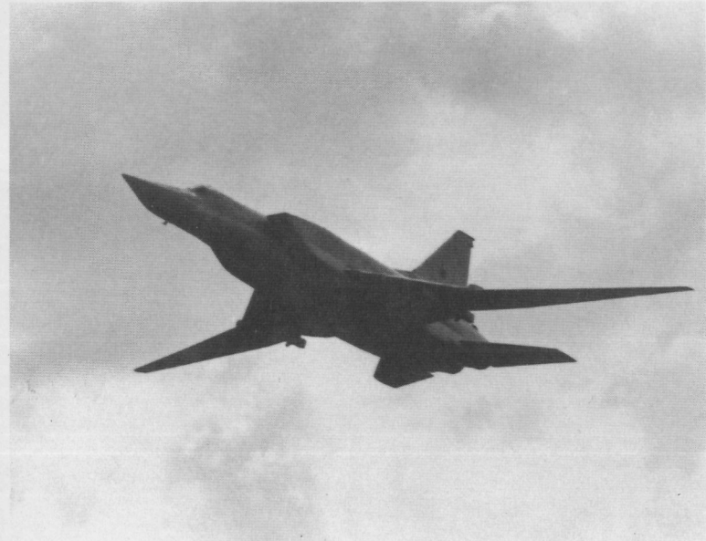
The most recent version of the Backfire is the Tu-22M3 Backfire C. This aircraft has a new attack/navigation radar as is evident from the change in the nose contours. It also uses chisel exhausts, similar in shape to those on the MIG-25 fighter. This particular aircraft has twin missile pylons for the AS-4 Kitchen.
