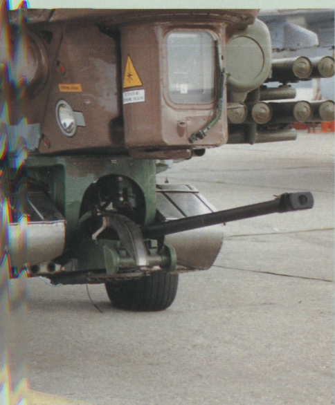
The 2A42 cannon on the Mi-28 has large silver heat shields on either side of the turret assembly.
