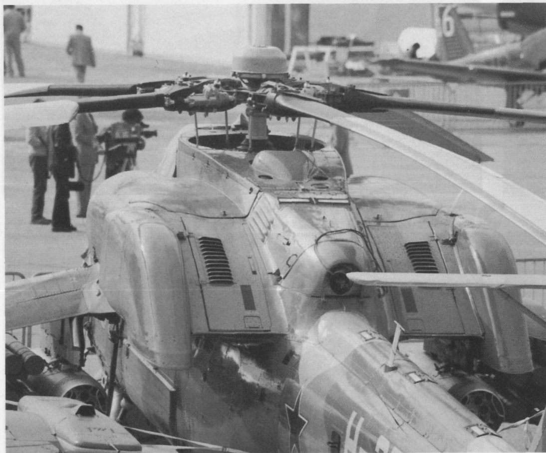
A close-up over the spine of the Mi-28 showing the rotor assembly and engine covers.
