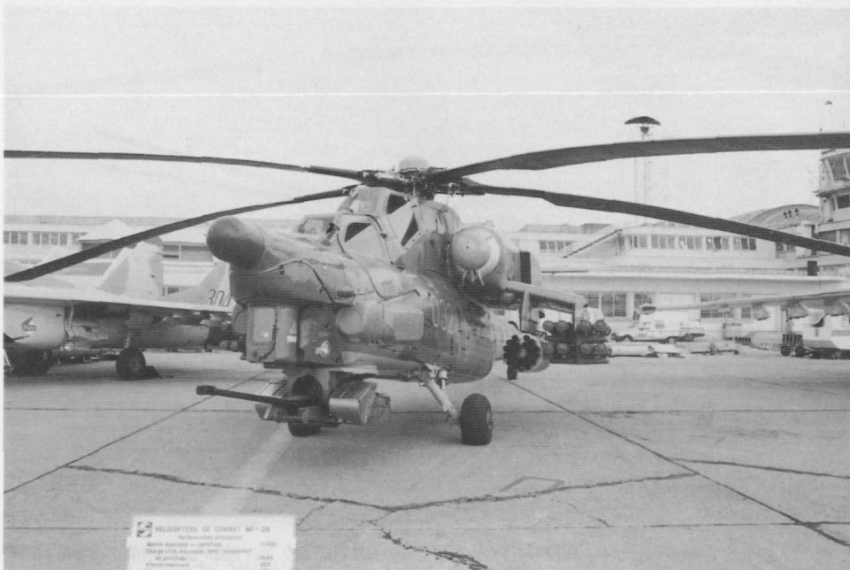
Another view of the nose of the Mi-28. This view emphasizes the 30mm 2A42 cannon, the S-8 80mm rockets and the eight Shturm (AT-6 Spiral) anti-tank missiles.
