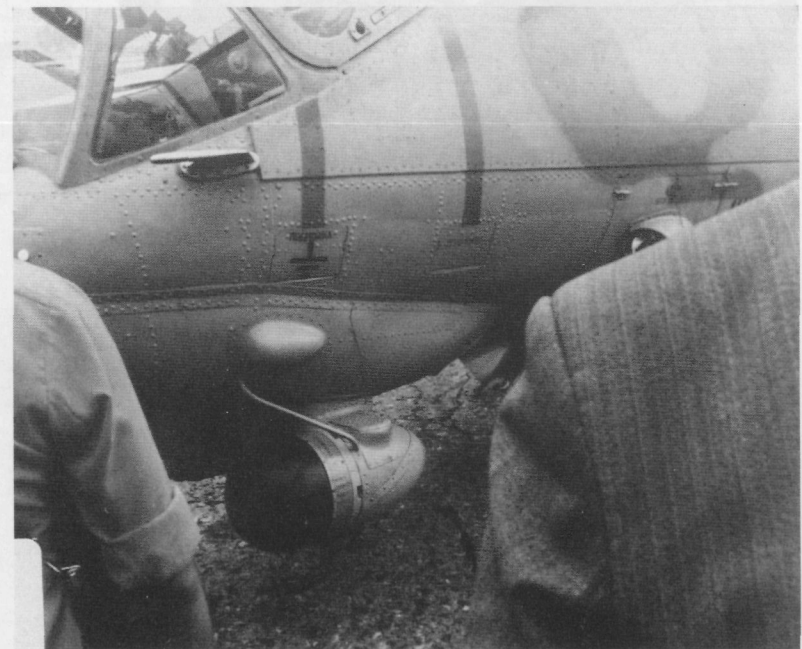
The 9M114 Shturm/AT-6 Spiral anti-tank missile requires a different command guidance antenna than earlier models, and is seen here in close-up.
