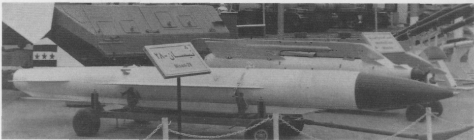
The S-24 is a large 240mm diameter unguided rocket fired from Soviet attack aircraft. This view shows a pair of S-24 of Iraqi manufacture, called the Nasser 240. (Christopher Foss)
