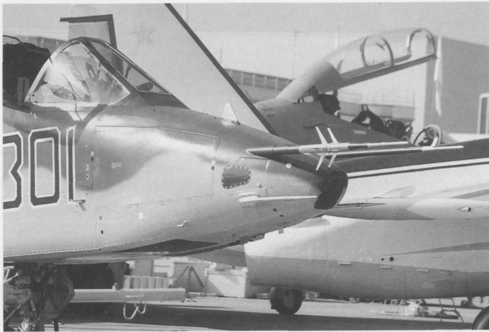
A close-up shot of the nose probes on the Su-25K. At the top of the nose is the Khrom Nikel IFF blade antenna.
