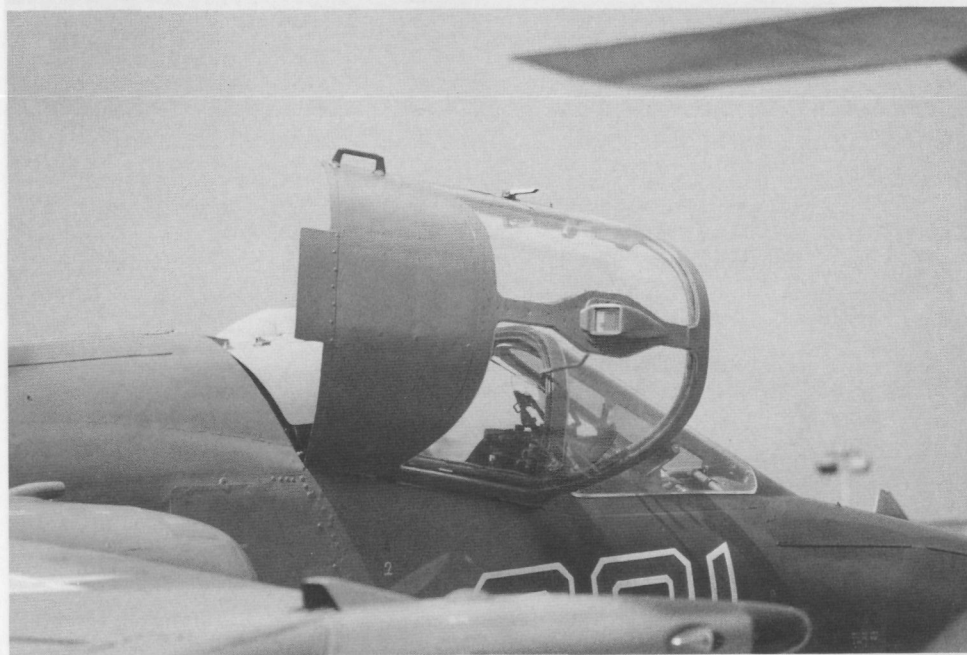
A close-up of the opened canopy. Prominent on the crest of the canopy is a small periscope, positioned to allow the pilot a view over the rear of the aircraft to watch for enemy fighters.
