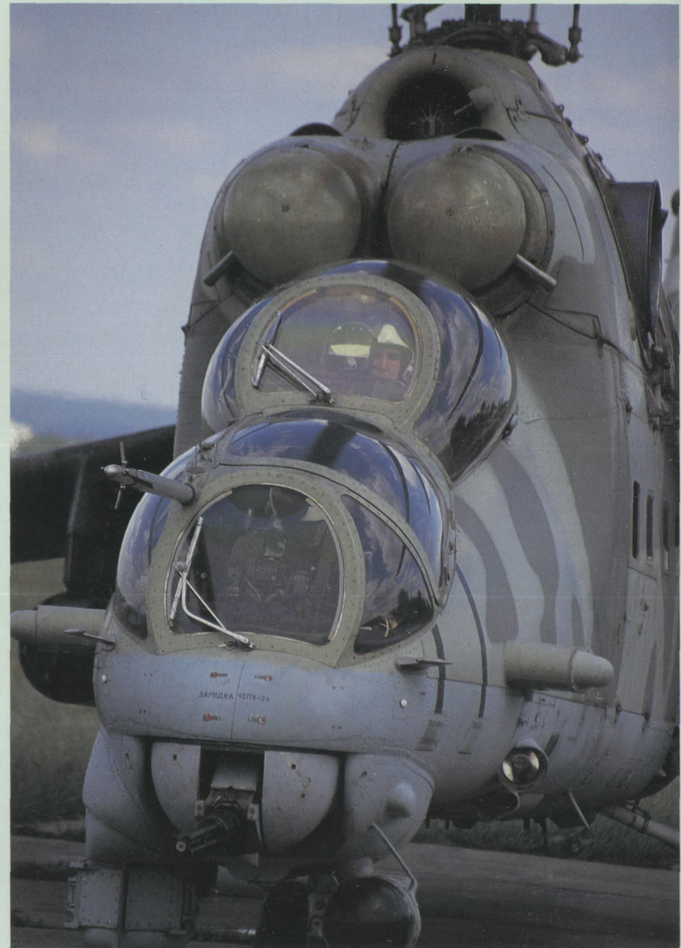
A nose view of a Czechoslovak Mi-24V of the 11th Helicopter Regiment. The nose stencilling reads: Zaryadka ChSPU-24, indicating the reloading point for the nose YaKB-12.7 machine gun. (Yves Debay)
