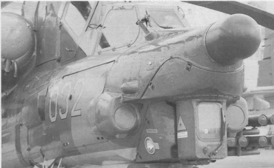
A close-up view of the nose of the Mi-28 Havoc. The production program of the Mi-28 has been delayed by slow development of thermal imaging night sights for the aircraft. As a result, the cheek mounted sights were blanked over at Le Bourget. The sight in the center turret is a daylight only sight for the gunner. The black nose dimple is the antenna cover for the guidance system of the Shturm missile.
