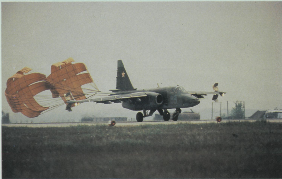
A Soviet Air Force Su-25K Grach landing with its braking parachutes fully extended. This particular aircraft has blue "bort" numbers. (Sovfoto)
