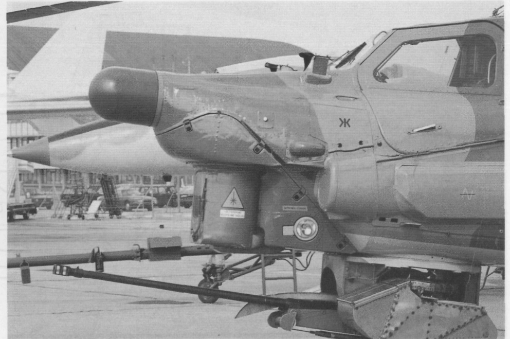
A profile view of the Mi-28 nose. The small searchlight folds outward during landing approaches. The 2A42 30mm cannon is a derivative of the weapons used on the BMP-2 armored vehicle.
