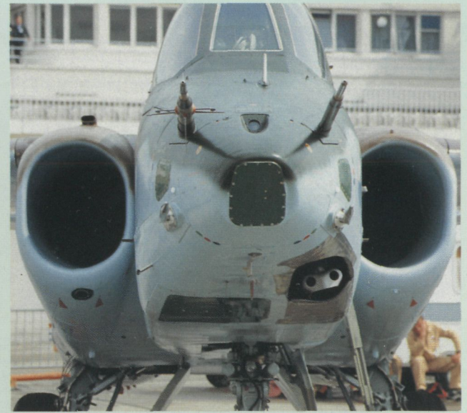
A close-up of the nose of Rutskoï's Grach. The front laser-ranger panel is covered by a protective green cover. This view shows the twin-barrel 30mm cannon to the right. The two nose probes are the ILS antenna to the left of the picture and the pitot to the right. Under the fuselage is a glossy dark green radar altimeter panel.
