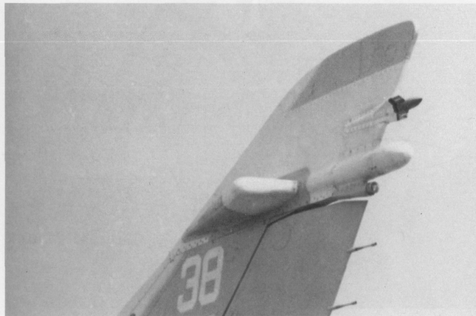
A view of the tail tip on the Khodynka Su-24M. The prominent fairings above the number 38 were first seen on the Fencer C variant and contain rearward pointing radar warning antennas. (Nick Cook)
