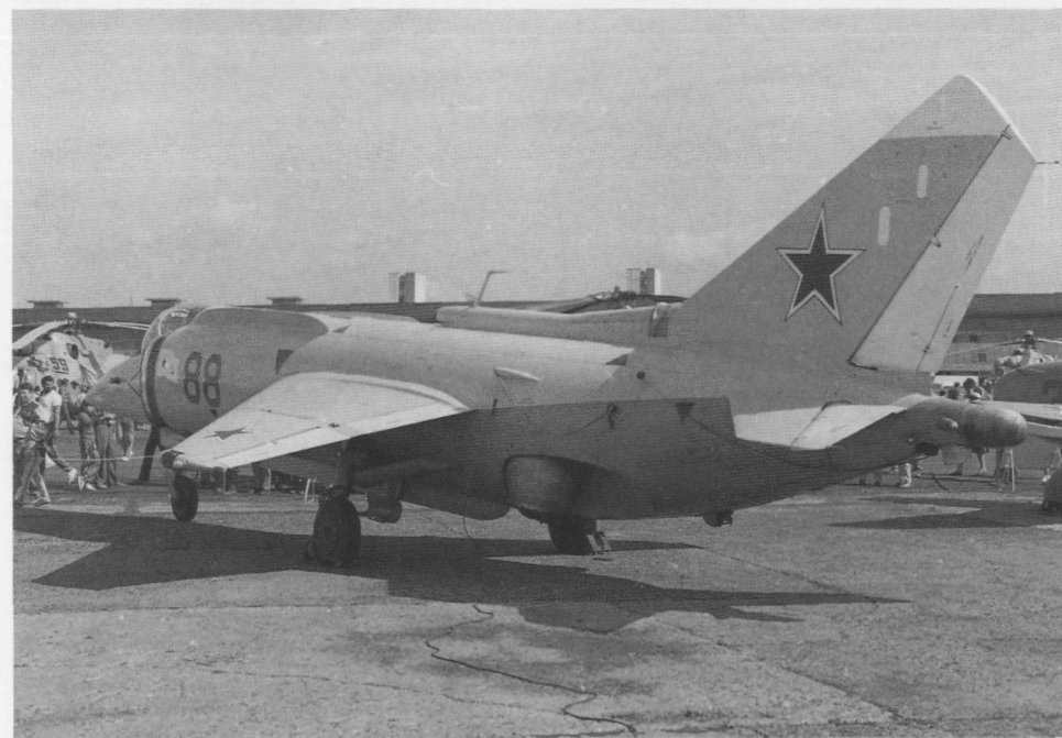
This Yak-38 displayed at Khodynka in 1989 carries the new naval paint scheme. The earlier scheme consisted of dark blue upper surfaces and dark green anti-corrosion paint on the undersides. The new scheme consists of light grey upper surfaces and the standard dark green undersides. (Nick Cook)
