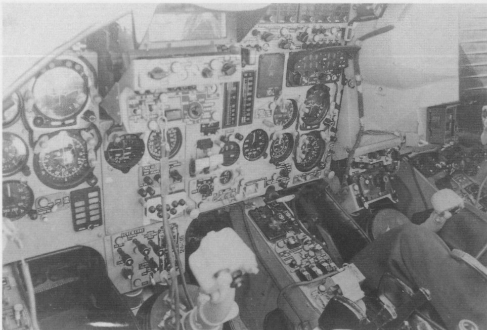
A cockpit interior view of the Su-24M Fencer D. This view shows the left side where the pilot sits.
