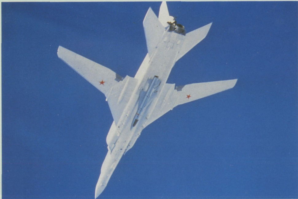
The primary armament of the Tu-22M2 Backfire B is a standoff missile, often the AS-4 Kitchen as seen in this view.
