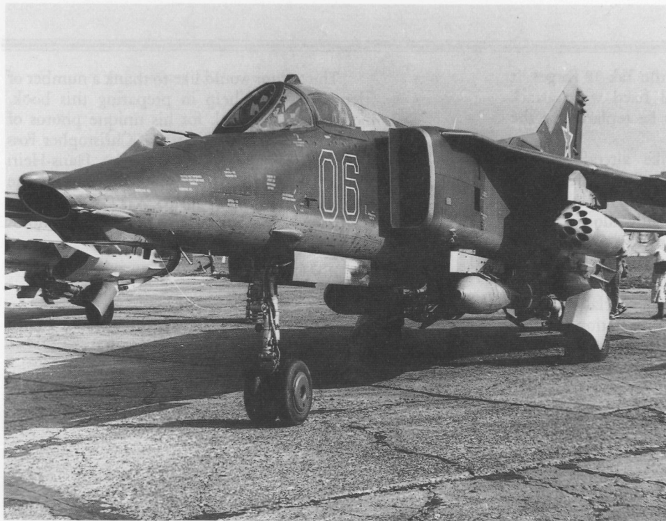
The MIG-27KR is the latest attack version of the Flogger family. It is most readily distinguishable by its longer nose and the oval optical port at its tip. This particular aircraft was exhibited at the Central Frunze Air Base at Khodynka in August 1989.
