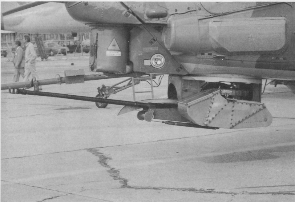
This gun configuration is peculiar to the third prototype. Earlier prototypes had a slightly different configuration with a ballistic housing over the gun.
