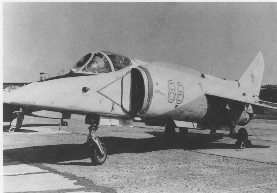
This Yak-38 displayed at Khodynka in 1989 carries the new naval paint scheme. The earlier scheme consisted of dark blue upper surfaces and dark green anti-corrosion paint on the undersides. The new scheme consists of light grey upper surfaces and the standard dark green undersides. (Nick Cook)
