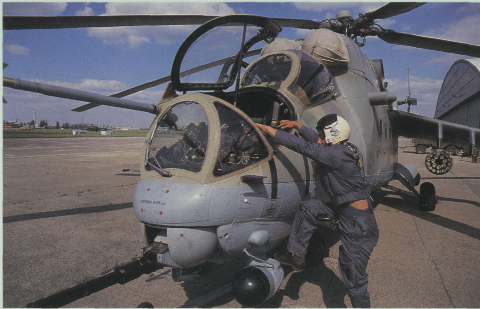
The weapon's systems officer of a Plzen 11th Helicopter Regiment Mi-24V boards his helicopter. His left foot is on the radio-command guidance antenna pod used to control the Shturm-V anti-tank missile. The sub pylon behind the cockpit area is for a missile-warning sensor, sometimes dubbed "the Natasha device". (Yves Debay)
