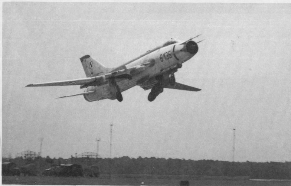
One of the less common versions of the Fitter family is the Su-20 Fitter C, seen here operating with a Polish Su-20 regiment near Pila. This aircraft was an evolutionary bridge between the fixed wing Su-7 and the latter variable geometry wing Fitters. (Wojciech Luczak)
