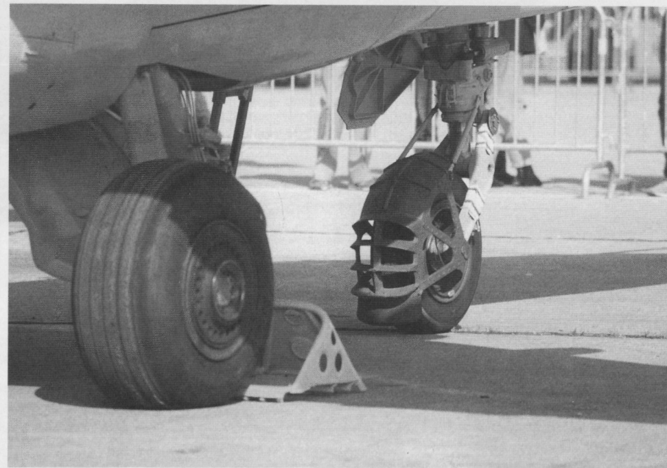
A rear view of the landing gear from the right, showing details of the anti-FOD debris catcher.
