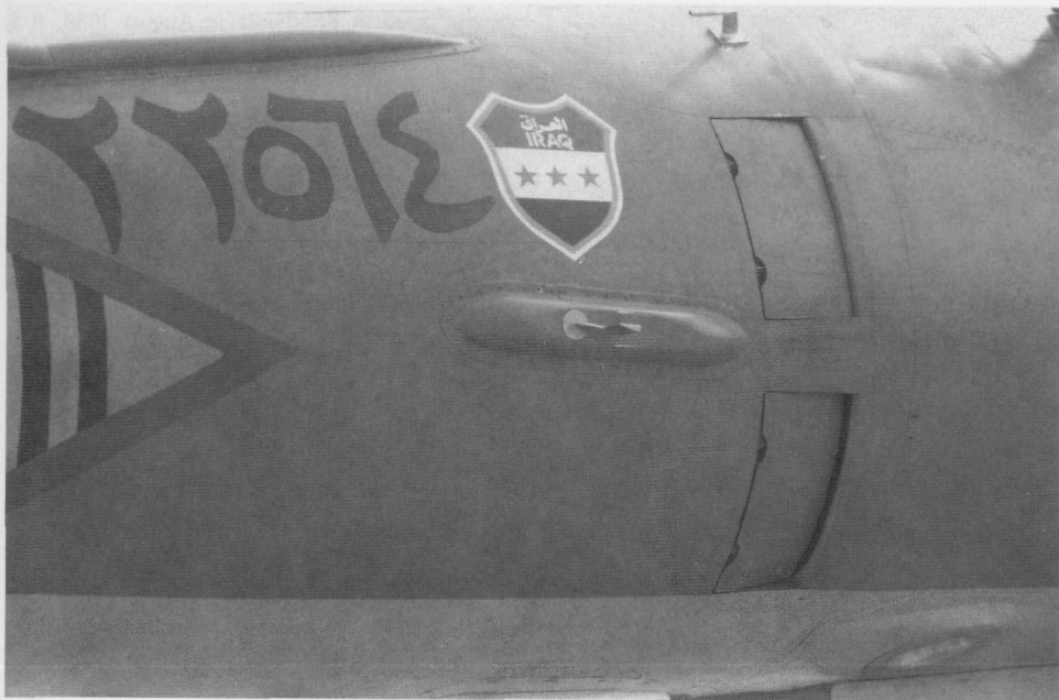
A close-up of the nose markings on the Iraqi Su-22. The shield insignia above the angle-of-attack sensor (in the same colors as the national flag-green, white, red and black) is occasionally seen on Air Force aircraft. The aircraft number, painted in black, is in Arabic: 22564. (Christopher Foss)
