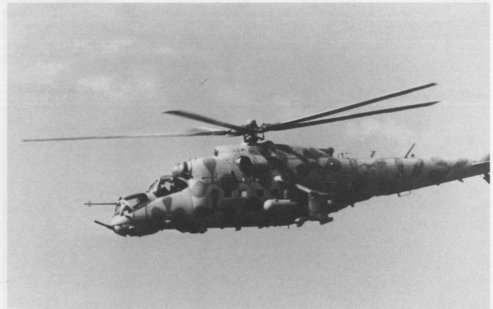
The most mysterious version of the Hind is the Mi-24R Hind G. It is basically similar to the Hind D, but lacks the missile armament on the stub winglets. It was originally believed to be chemical detection variant, but is now believed to be an electronic warfare type. The devices on the wing-tip may be configured for this role.
