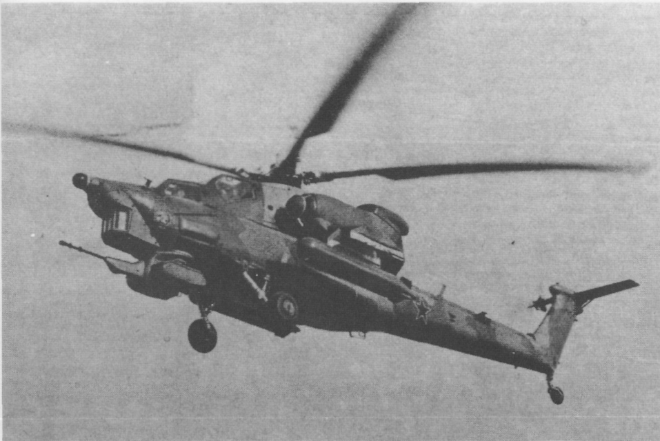
A right side view of the Mi-28. The pilot sits in the upper rear station, the gunner in the lower forward station.
