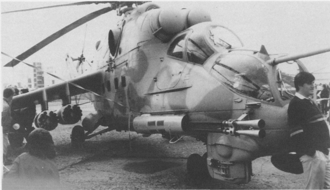
The latest armament variation on the Mi-24 family is the Mi-24P, armed with a twin GSh-30-2 30mm cannon in place of the usual YaKB-12.7.
