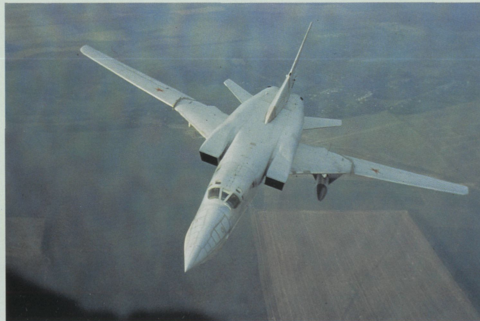
A nose-on view of a Tu-22M3 Backfire C bomber showing the characteristic features of this variant: the high speed air intakes and new nose. (Sovfoto)
