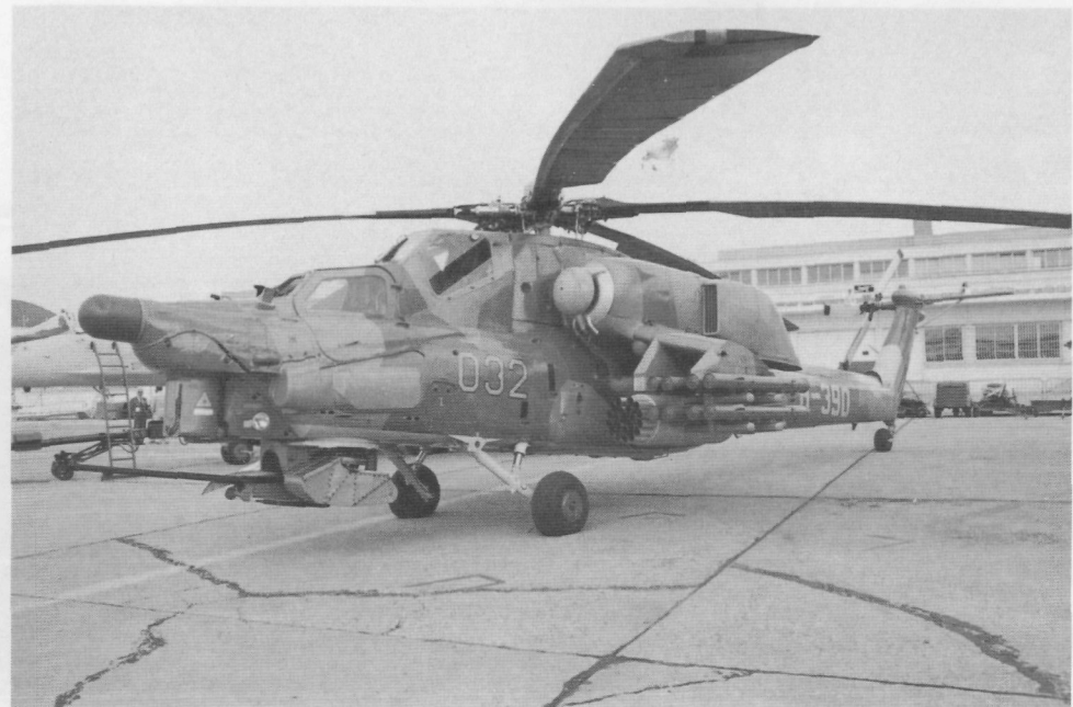
The side profile of the Mi-28 is considerably sleeker than the older Mi-24 since it lacks a center troop compartment.
