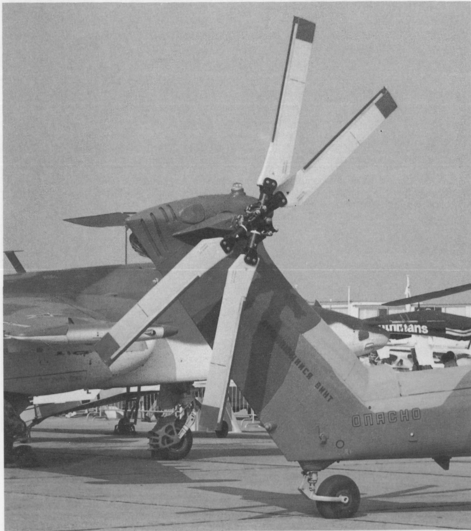
A detail shot of the rear tail rotor assembly of the Mi-28. This is in overall grey with red tips and black leading edges.
