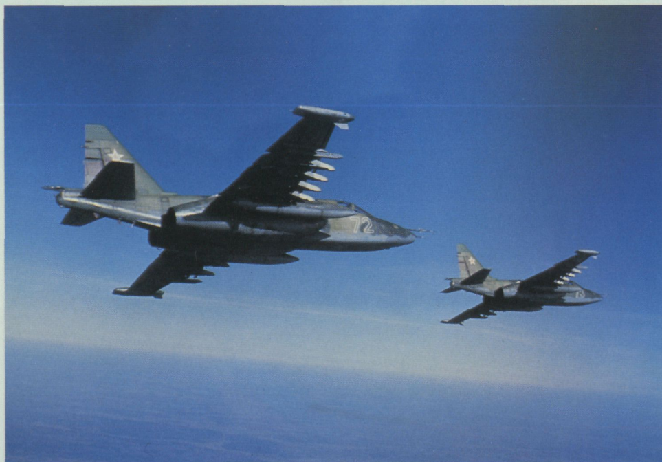
A pair of Su-25K on a practice mission. The aircraft uses subdued "bort" numbers, simply a hollow white stencil with no interior color. (Sovfoto)
