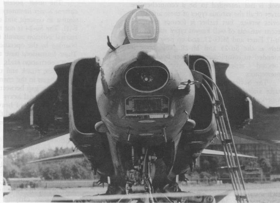
A close up of the nose of the MIG-27KR. The two optical ports contain a trainable laser designator for guiding laserguided bombs and missiles and an electro-optical sight for night attack missions.
