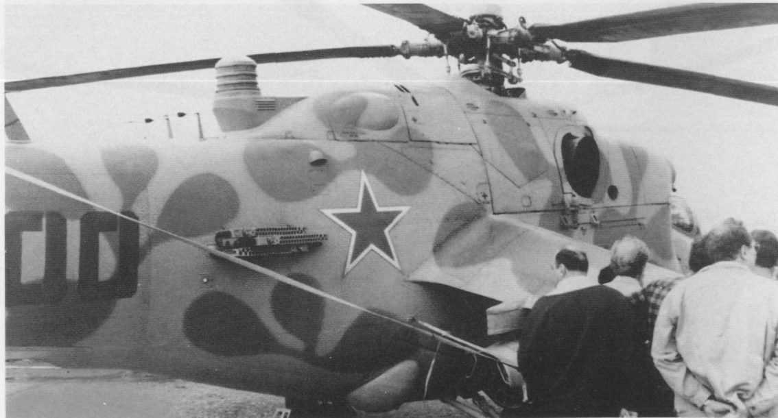
The combat experience in Afghanistan against heat-seeking anti-aircraft missiles has led to a number of antimissile countermeasures. This Mi-24VE has the later ASO-3 configuration, with the flare dispensers mounted on the fuselage side (behind the star). On the fuselage spine behind the rotor is the prominent "Hot Brick" system, used to confuse the sensor in heat-seeking missiles. This aircraft is not fitted with the usual hot-gas diffuser normally fitted over the exhaust pipes.
