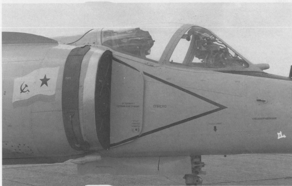
A close-up of the nose of the Yak-38. The warning markings are in red. Although the Yak-38 resembles the Harrier, the engine configuration does not permit thrust vectoring. The Yak-38 is not a popular aircraft in service due to its high accident rate. (Nick Cook)
