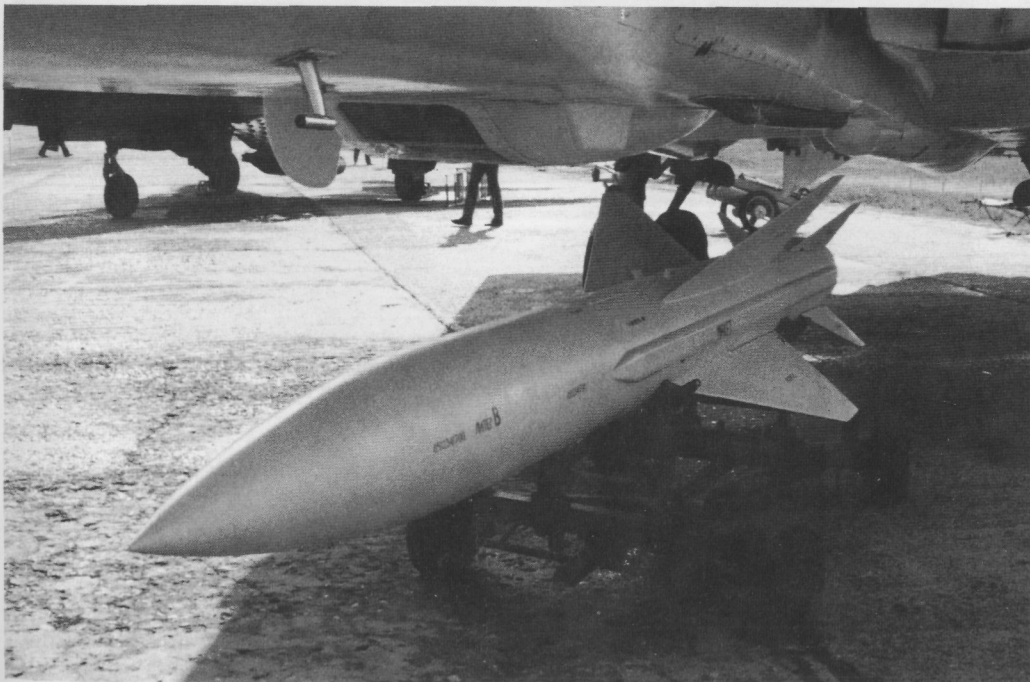
▼ A close-up view of an AS-11 Kilter anti-radar missile as displayed at Khodynka under an Su-24. Above the missile can be seen the electro-optical guidance station added to the Su-24M Fencer D series for guiding advanced precision-guided missiles and bombs. (Nick Cook)
