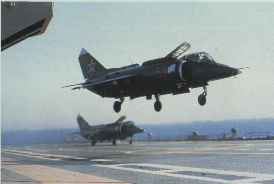
A pair of Yak-38 naval strike aircraft aboard the light carrier Novorossisk. The Yak-38 is considered to be an attack aircraft, rather than a fighter by the Soviet Navy. (Sovfoto)
