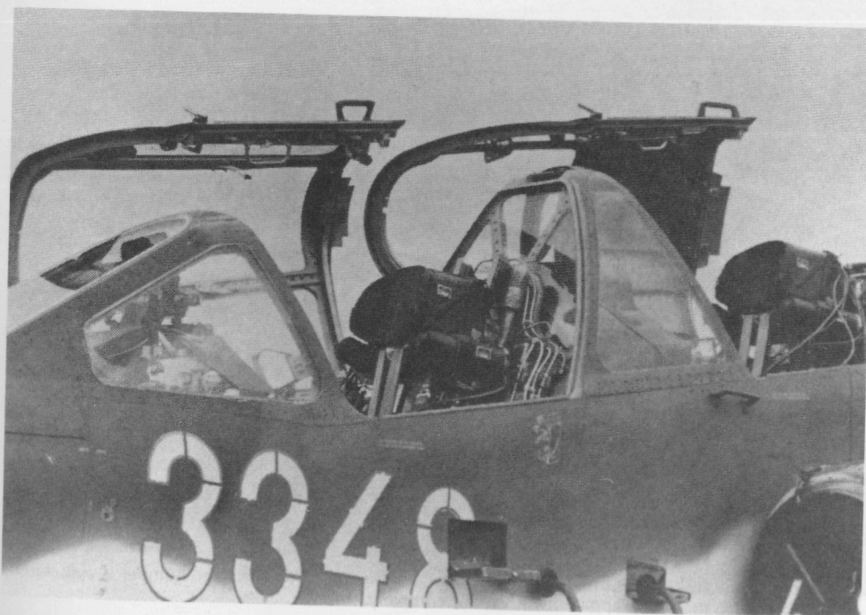
This photo of an Iraqi Su-25K clearly shows the differences with the modified Afghanistan aircraft. Note the lack of the air intake and ASO flare dispensers. (Christopher Foss)
