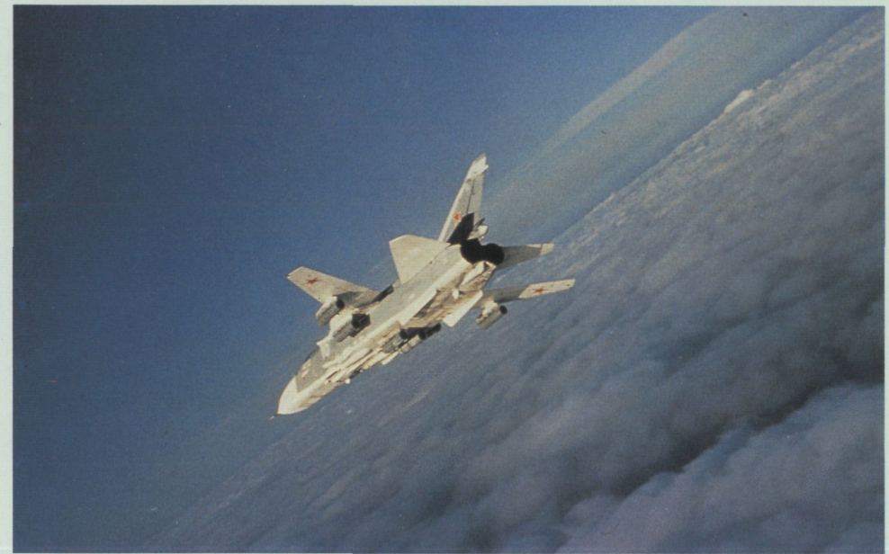
An Su-24M Fencer D on a peacetime training mission armed with S-5 57mm rocket pods. These pods are commonly used in peacetime training, though in combat, the Su-24 would more commonly be used with more sophisticated ordnance. (Sovfoto)
