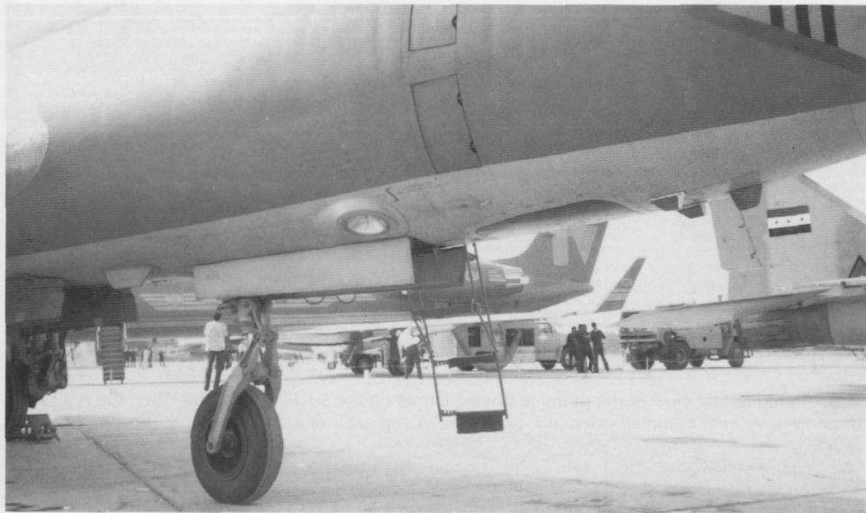
A detail view of the nose of the Su-22M4. At the front corners of the landing gear door are two landing searchlights. Forward of these is a dark green dielectric panel for the radar altimeter, preceded by two unidentified antennas and a Khrom-Nikel IFF blade antenna. (Christopher Foss)
