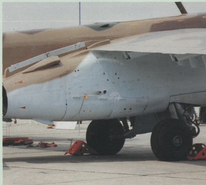
This photo of the mid-section of the aircraft shows the large bay doors over the engine, developed to allow the aircraft to be easily serviced in the field.
