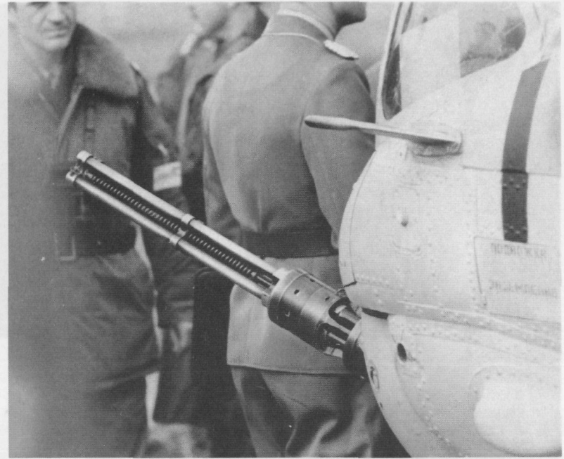
A close-up of the barrel of the YaKB-12.7 machine gun on the nose of the Mi-24D.
