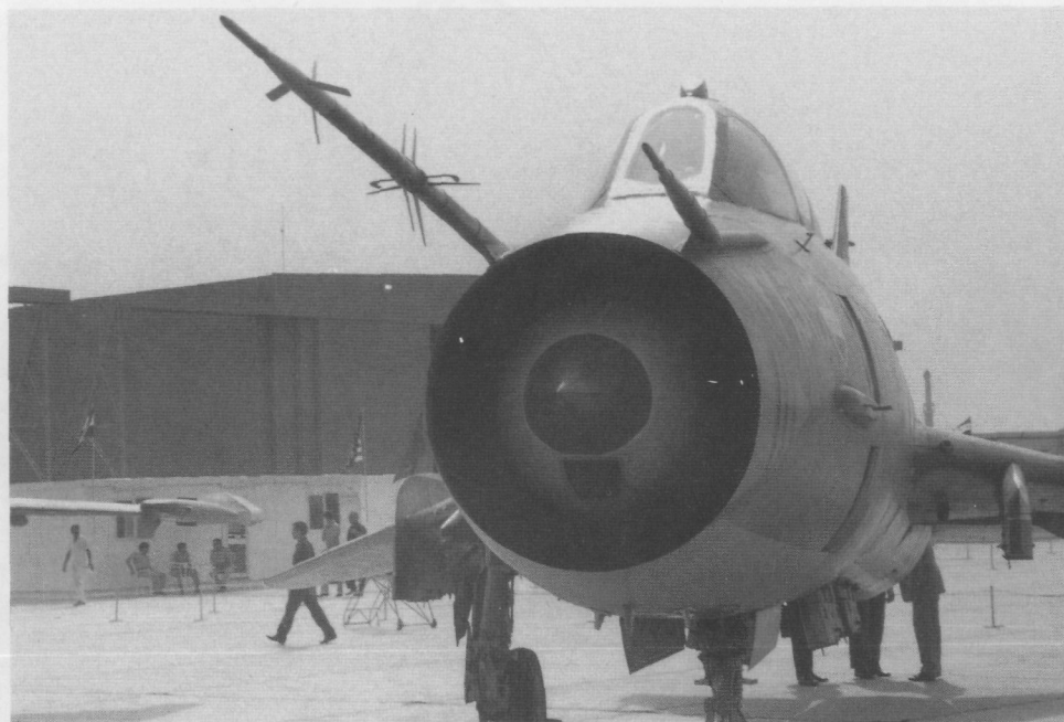
A view of the nose of the Su-22M4. The air intake cone is silver with a green-dielectric plastic tip. The small optical port on the lower side of the cone contains a laser range-finder. The large probe over the intake has an angle-of-attack sensor and the antennas for an instrumented landing system. (Christopher Foss)
