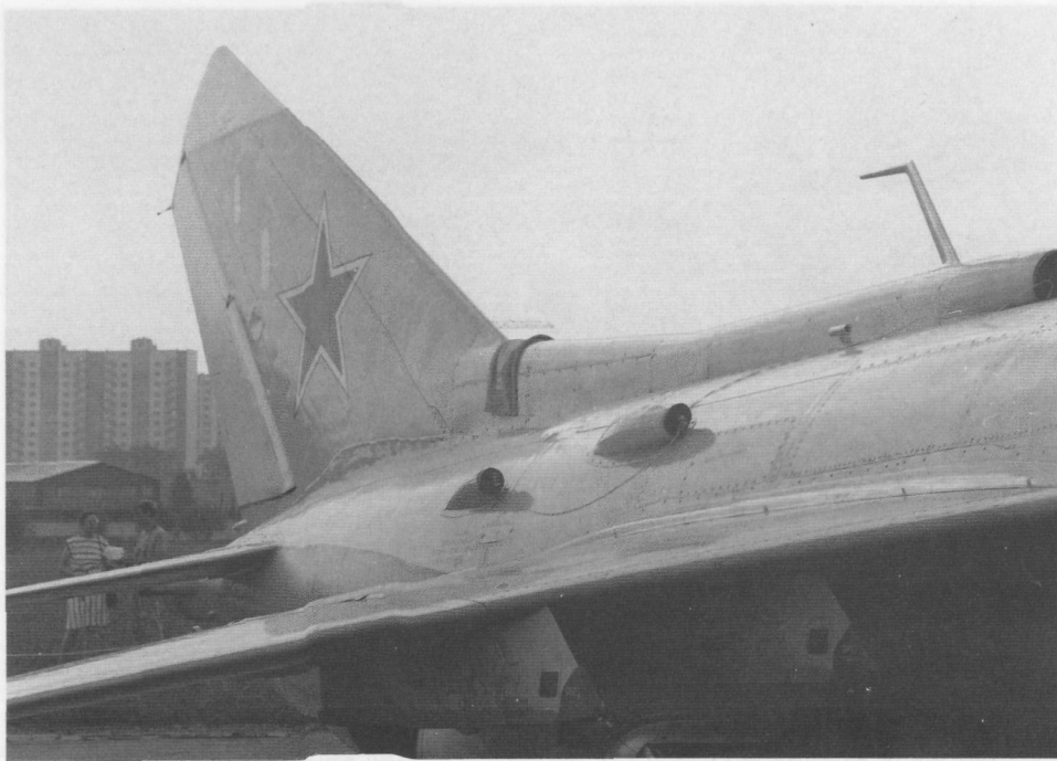
A detail view of the Yak-38 upper rear fuselage showing the two wing pylons in the foreground. (Nick Cook)
