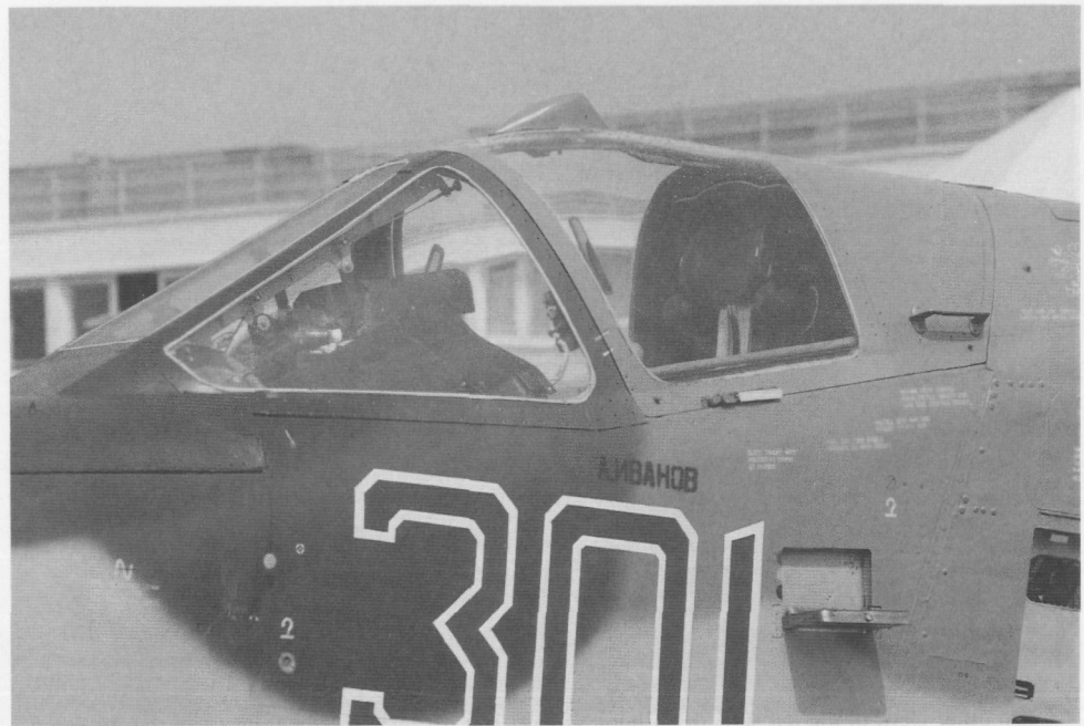
A close-up of the Su-25K canopy. The Su-25 has a much smaller gun sight than the HUDs fitted to contemporary Soviet fighters, and so has better vision from the canopy.
