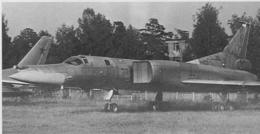
The prototype of the Tu-22M1 Backfire A differed from the production Tu-22M2 Backfire B in a number of details including the larger rear brake fairing on the tail and the under-nose attack sensor. The prototype was designated Tu-126, which has led to the Backfire sometimes being mislabeled as the Tu-26.
