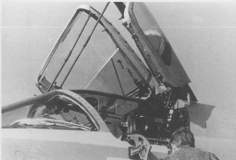
A view of the Su-24M cockpit with the canopy open.
