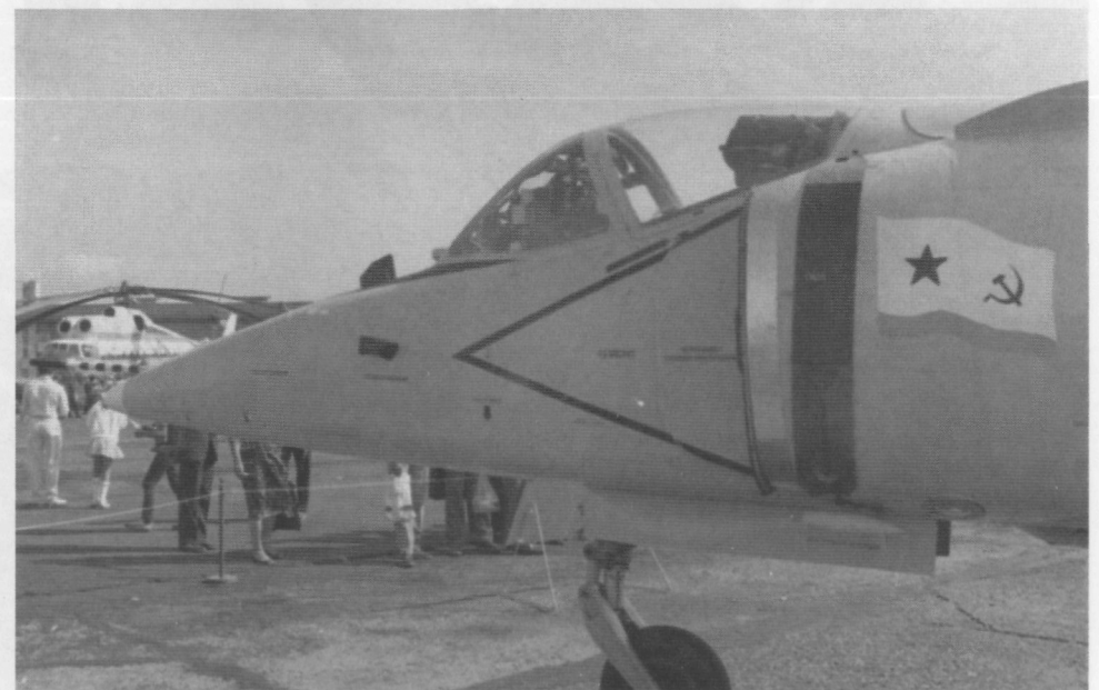
A detail view of the left side of the Yak-38. The antenna in front of the cockpit is the new style Khrom-Nikel IFF. (Nick Cook)
