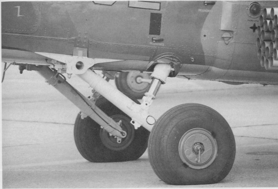
A close-up of the landing gear. The Mi-28 gear has been designed to withstand crash shocks, based on experiences of Mi-24 crashes in Afghanistan.
