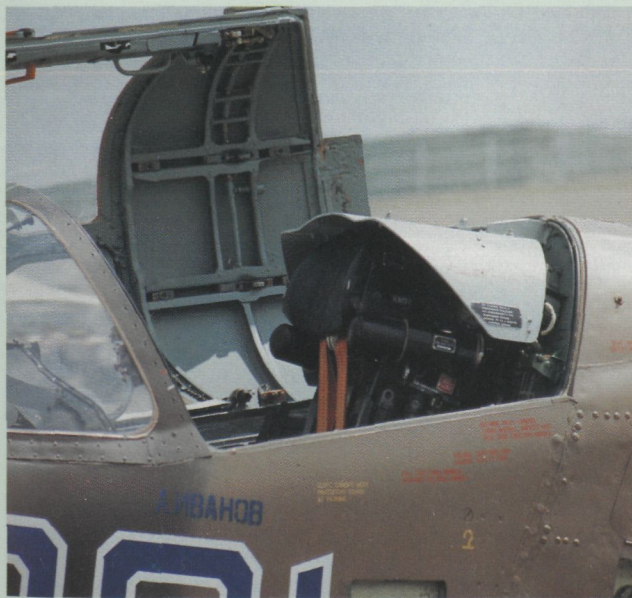
The Su-25K is fitted with a Severin K-36 ejection seat (as in the MIG-29 and Su-27). However, it is fitted with a panel of protective armor over the headrest for additional protection.
