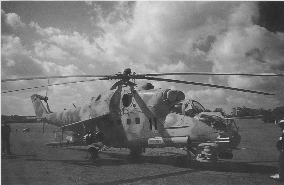
The Mi-35P displayed at Helitech in Britain in 1989. This is an export version of the Soviet Mi-24P and is armed with a pair of 30mm cannon in place of the usual turret armament. (Peter Wernli)
