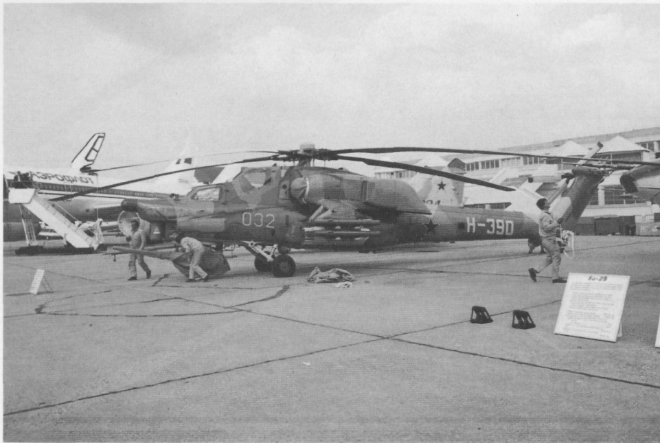
The Mi-28 has undergone evolution during its development, this view showing the first prototype with a different exhaust diffuser, different electro-optical nose sensor package and modified gun package.
