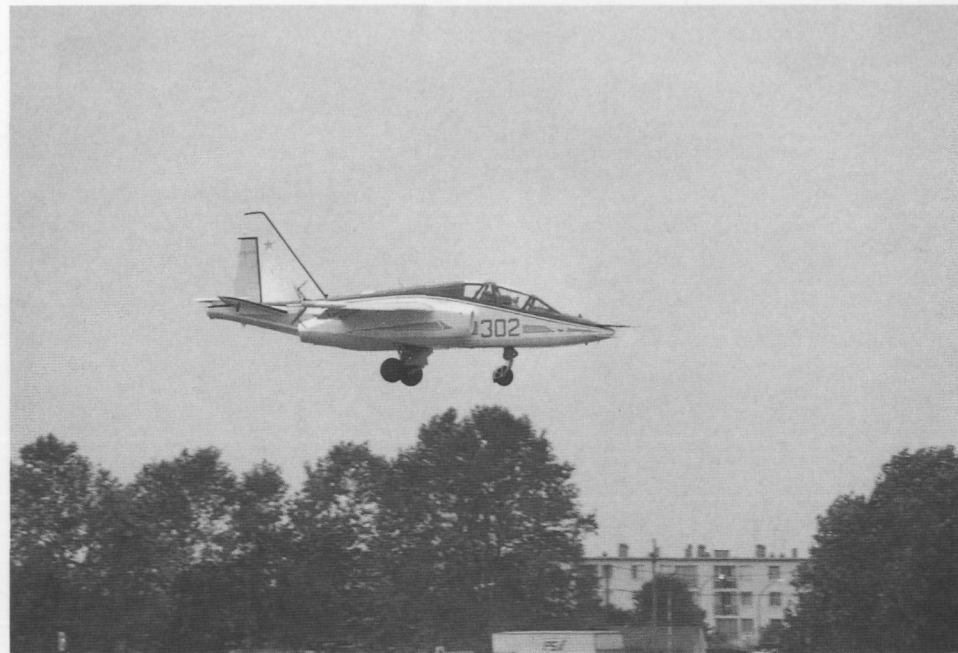
A Su-28 comes in for a landing at Le Bourget. The dive brakes at the ends of the wing pods are extended to bleed off speed.
