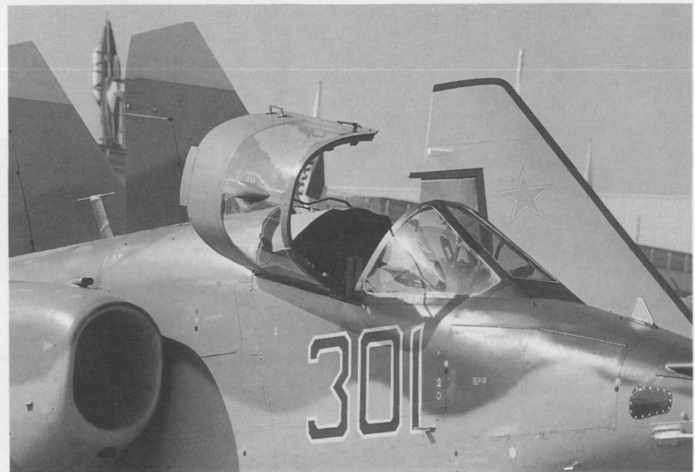
A view of the right fuselage nose with the canopy open.
