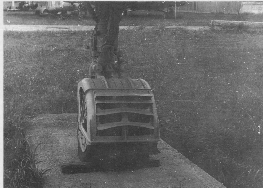
Another detail view of the anti-FOD device on the T-6 prototype at Monino, and similar to that on the current production aircraft.
