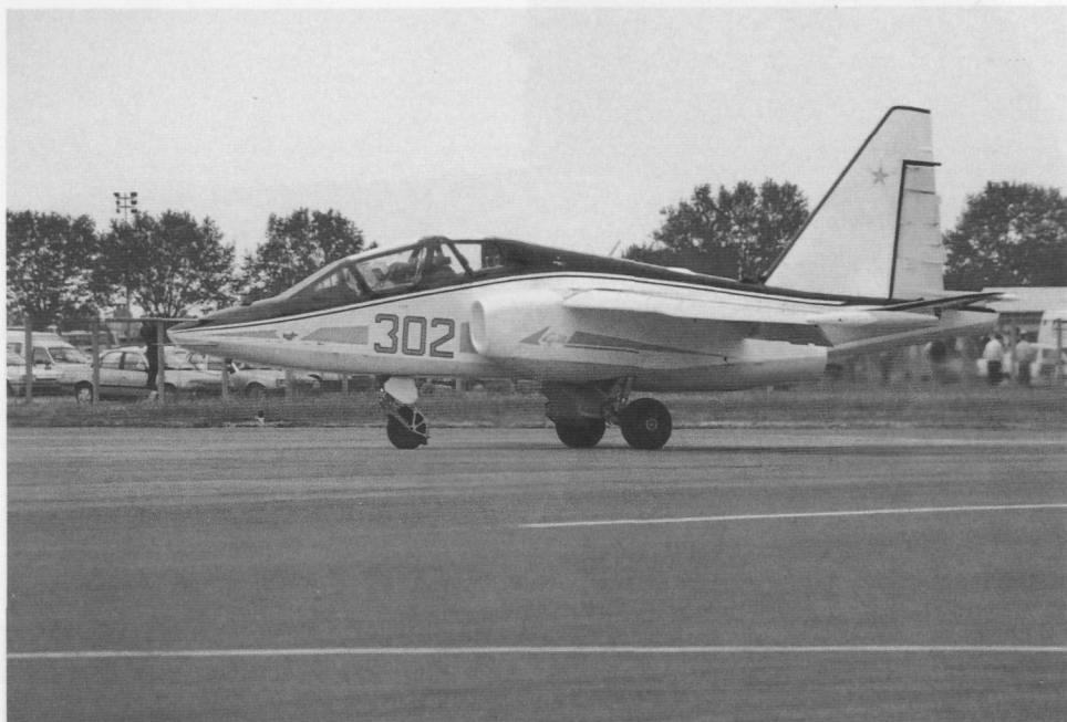
The Su-28 is an unarmed trainer version of the Su-25, and is also sometimes called the Su-25UT. It is intended to replace L-39 Albatross trainers in DOSAAF flight schools. The scheme here is for the DOSAAF schools.
